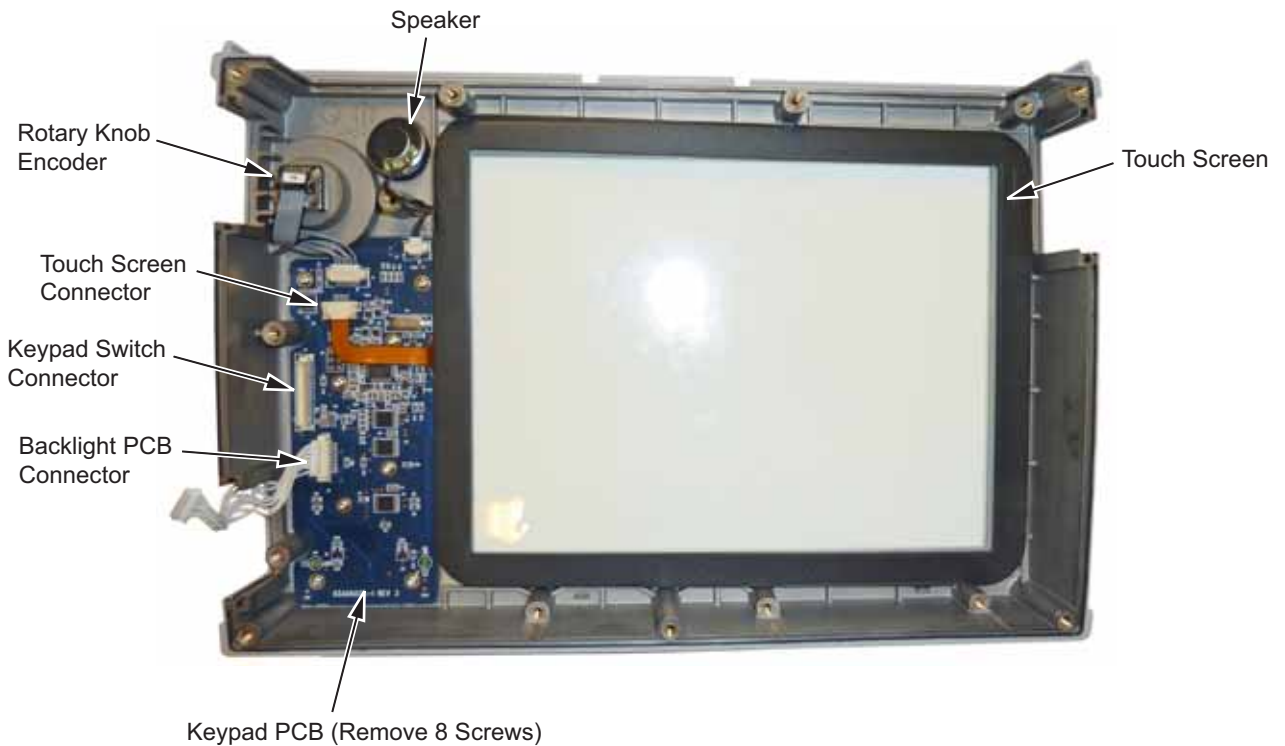
Figure 6-14. Front Panel Keypad Bezel
